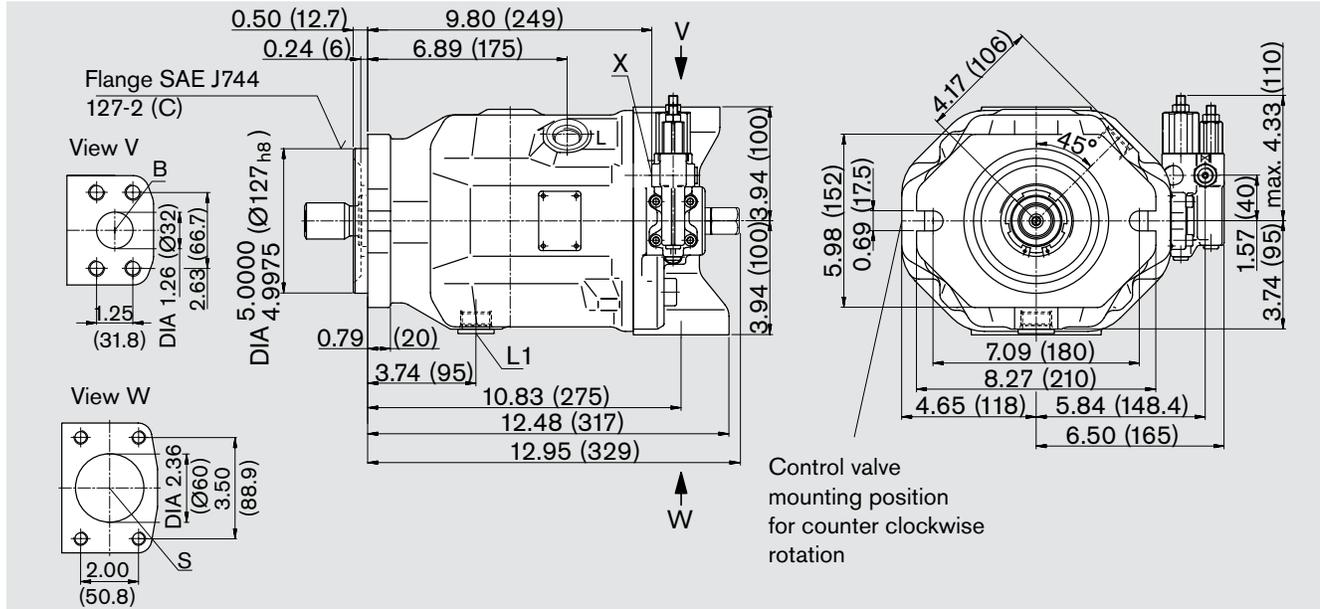
Control valve mounting position for counter clockwise rotation
