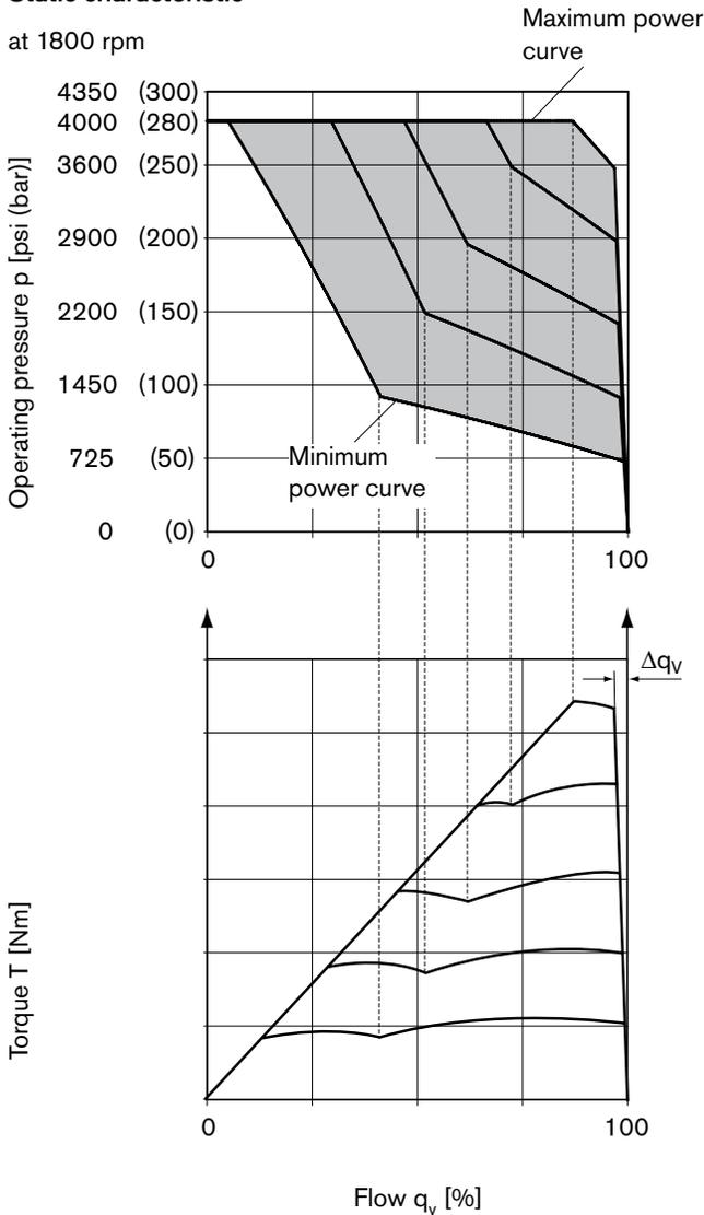
The power characteristic is set at the factory, please state your requirements in clear text e.g. 27 HP (20 kW) at 1800 rpm.
