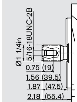
**R** Splined shaft 1 1/4 in 14T 12/24 DP<sup>4)</sup> SAE J744 - 32-4 (C)
